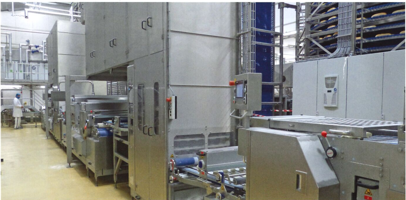
++ There are several König plants, e.g. an Industrie Rex AW with a KGN proofer for sandwich bread rolls
