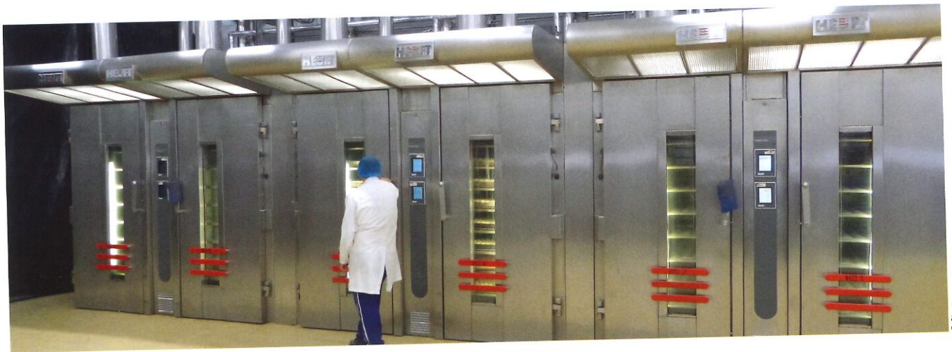
++ As well as rack ovens, there is also a Heuft multi-deck tunnel oven with thermo-oil and stone plates
