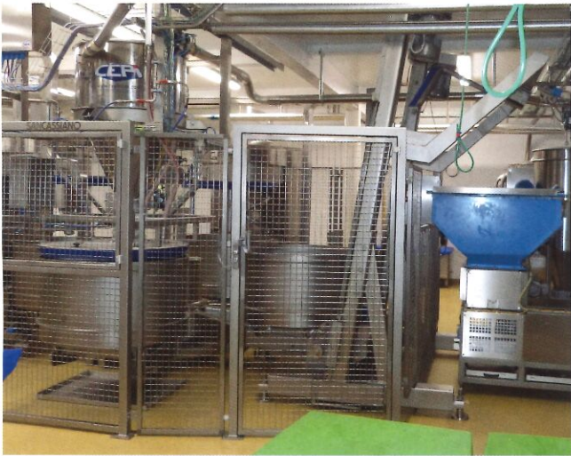
++ A Saccasiano mixer carousel automatically supplies wheat doughs to the lines. There is also a mixer for small dough batches
