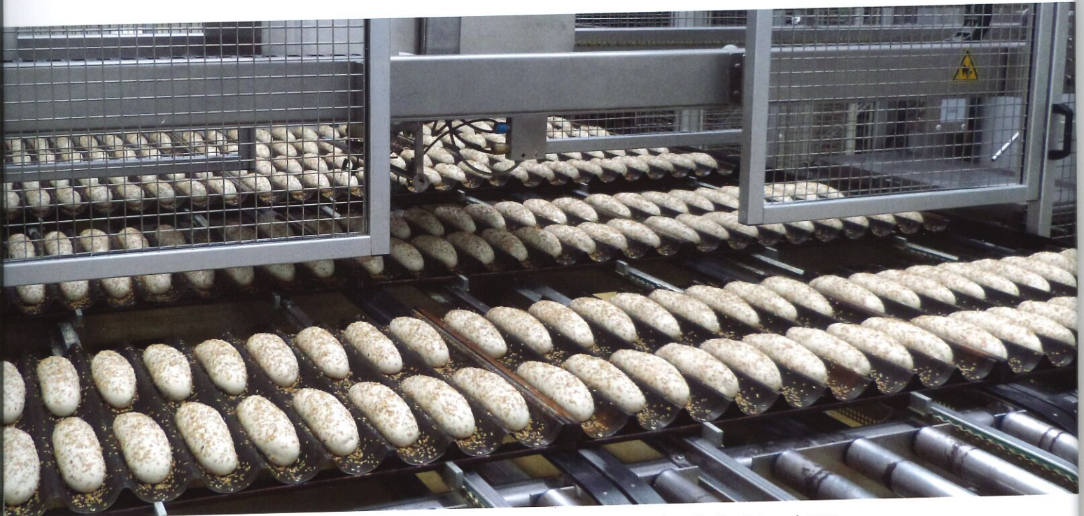
++ The dough pieces are strewn with seeds, automatically scored, then transported into the Heuft tunnel oven
