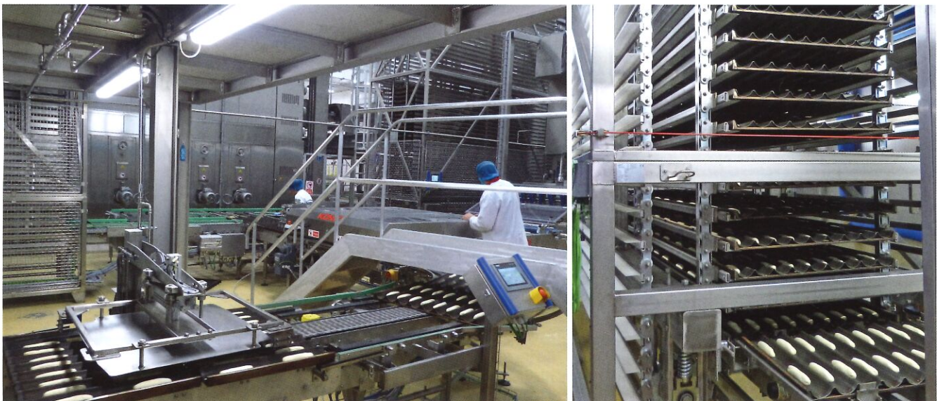
++ The dough pieces are deposited onto Diane coated trays. This is followed by the proofing process, including in a GBT paternoster proofer
